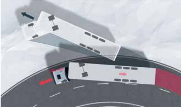
ESP compensatory braking when vehicle is oversteered
