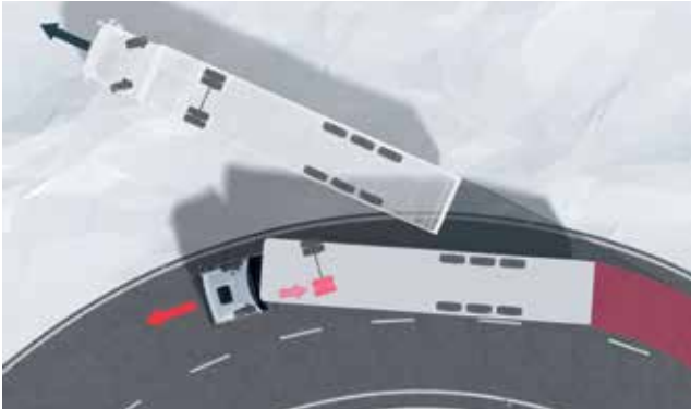
ESP compensatory braking when vehicle is understeered
