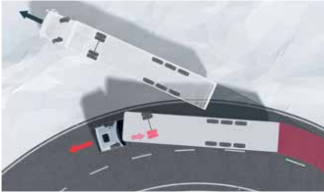
ESP compensatory braking when vehicle is understeered
